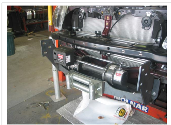
Figure 7: Warn XP9.5 fitted to winch frame.
